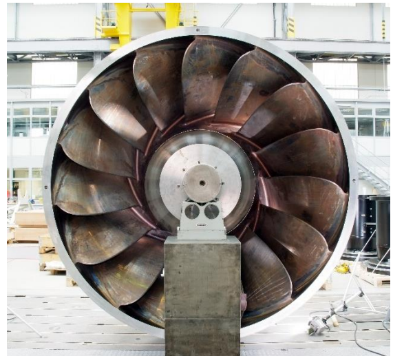
Figure 2: Voith Hydro Francis turbine during manufacturing [2]
