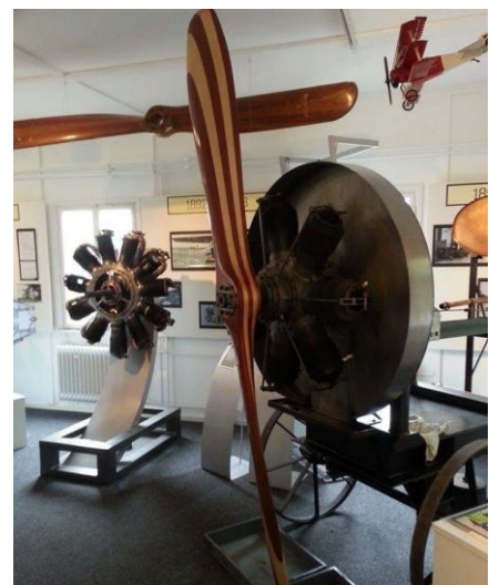
Figure 1: A restored revolving cylinder aero engine manufactured in Oberursel. The rotor is fixed to the casing therefore the cylinders are rotating allowing the idle stroke.
